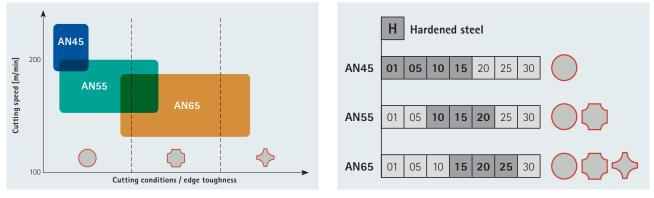
The new PCBN grades minimize chipping of PCBN tool edges by the strong bonding effect of proprietary CBN powder processing technology. And show reduced crater wear due to new developed ceramic binder systems which increased the hardness and heat resistance. The products are designed for processing various heat-treated steel parts and will provide improved workpiece surface quality and tool life.
